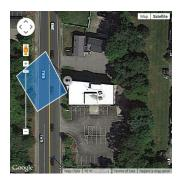
Geo-fences define the Field of View (FoV) for each camera. To draw a Geo-fence, place the camera by clicking on the map. Then click on spots on the map to define the area the camera can "see."
